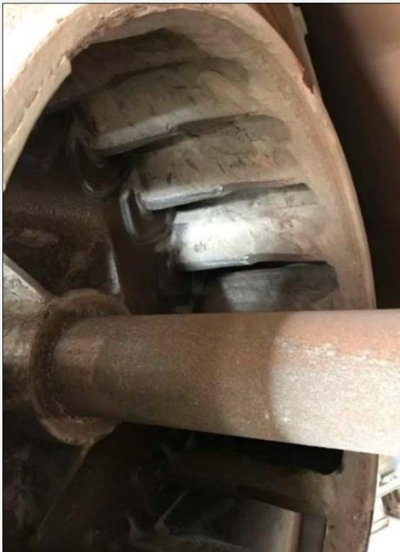
*New Turboimpeller with radial blades*
